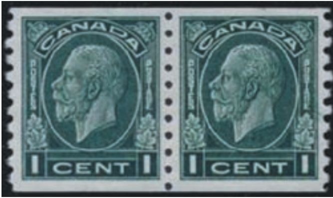
Canadian Stickney rotary press coil stamps perforated 8.70 vertically by a bar perforator.
