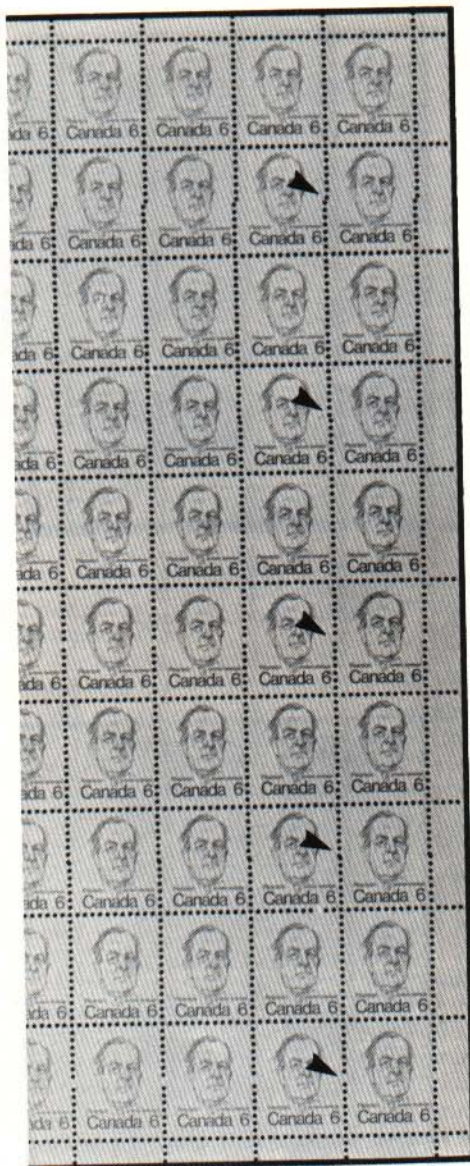
Fig. 9. CBNC 1 row T comb perforation. The arrows indicate the pronounced misalignments in the even rows only.
