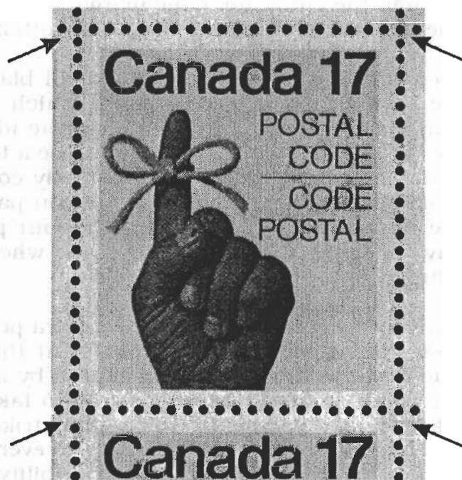
Figure 2. Wide and narrow "teeth" caused by misalignments between strikes of the 1-row T-comb perforator.
