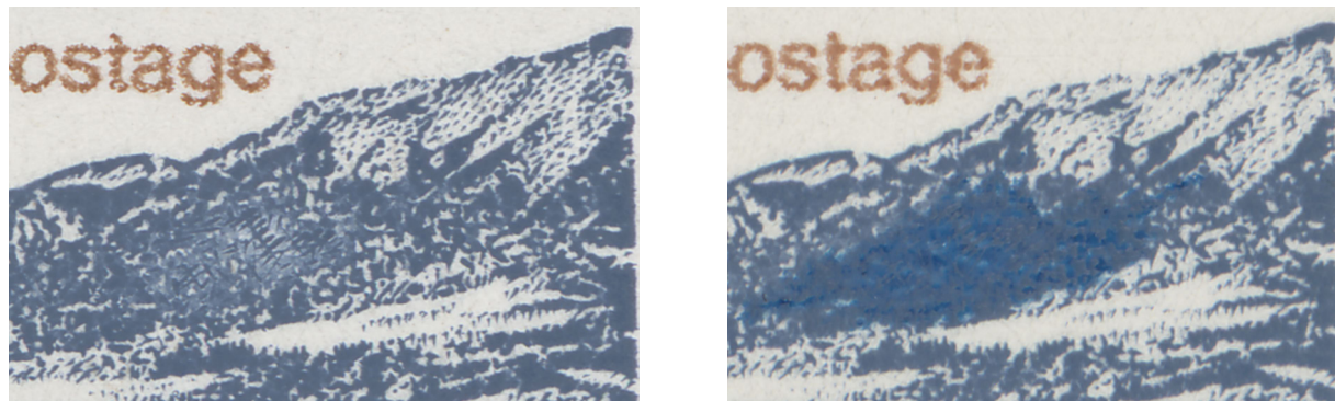
Figure 4. 15¢ design changes. Blue photogravure cylinder: blue added to mountains to improve opacity.
