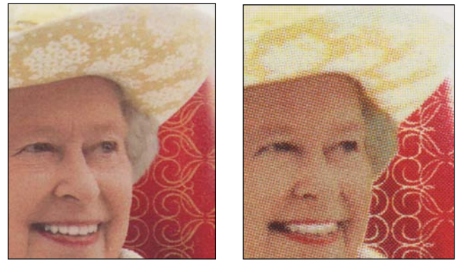
Figure 4. The detail on the Queen's face, hat, and background on the genuine (left) contrast with the rows of dots formed by the mesh screen on the counterfeit (right).
