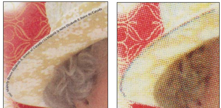
Figure 6. The microprinting on the genuine QE II stamp (left) is a bunch of blue and red dots on the counterfeit (right).
