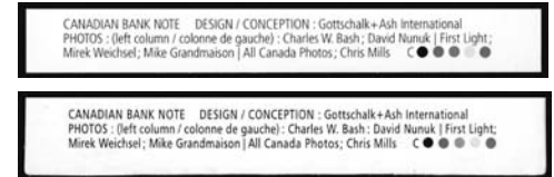
Figure 10. On the genuine Lighthouse booklets (top), the legend has a semi-colon after “Bash” and a space before the semi-colon at the end of the second line.
