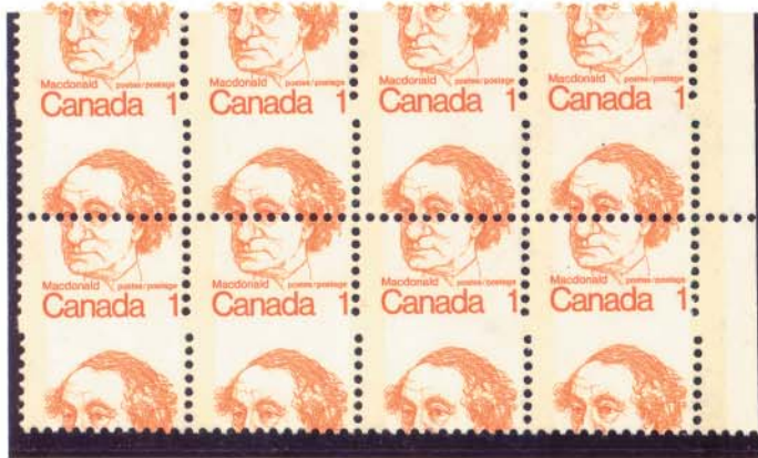
MISPERFORATION AND SHIFT SHOWING USE OF SINGLE "H" COMB PERFORATOR
